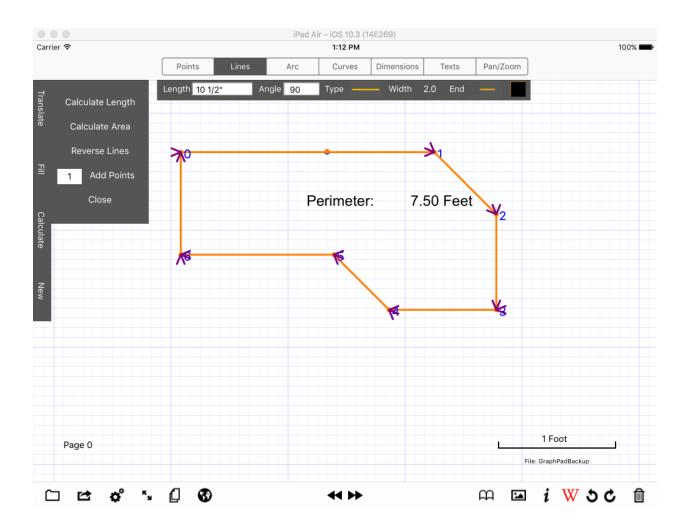
The New Points Tool is used to create a new line at the precise distance and direction for an existing point. To create a new line, select an existing point, use the tools buttons to set the precise distance and angle and press the "New Line" button. A new line will be created and the end point automatically active so users can quickly create the lines around the perimeter of an object.
